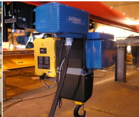
Flex 8EX used on Demag DC Pro
