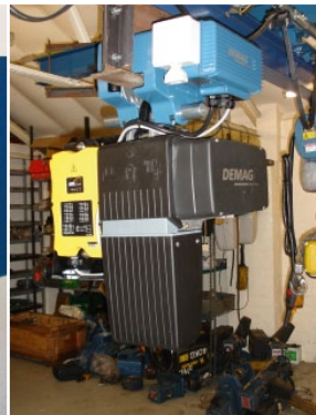
Flex 8EX used on Demag DC Com
