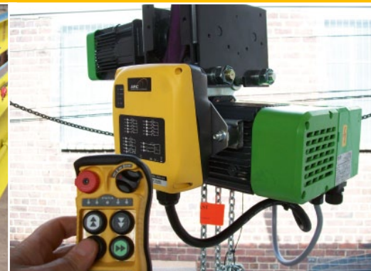
Flex 4EX used on Stahl chain hoist
